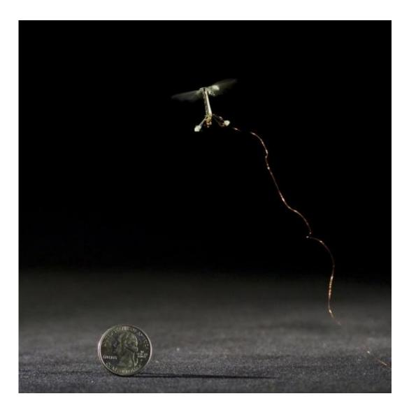
Inspired by the biology of a fly, with submillimeter-scale anatomy and two wafer-thin wings that flap almost invisibly, 120 times per second, this tiny robot not only represents the absolute cutting edge of micromanufacturing and control systems; it is an aspiration that has impelled innovation in these fields by dozens of researchers across Harvard for years. Credit: Kevin Ma and Pakpong Chirarattananon, Harvard University.
