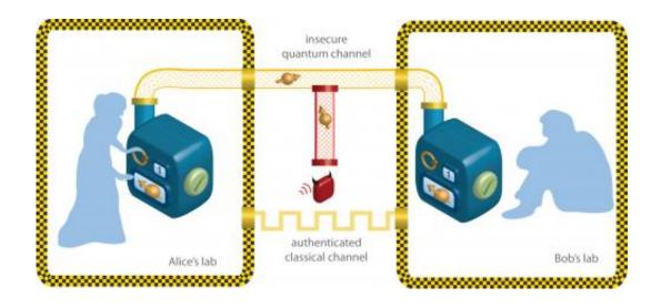
This image illustrates the standard assumption made in quantum cryptography, namely that the devices, such as photon sources and detectors, used by the honest parties, "Alice" and "Bob," are completely trusted (yellow boxes indicate the trusted region), whereas the channel connecting Alice and Bob may be controlled by an adversary. Credit: Renato Renner.
