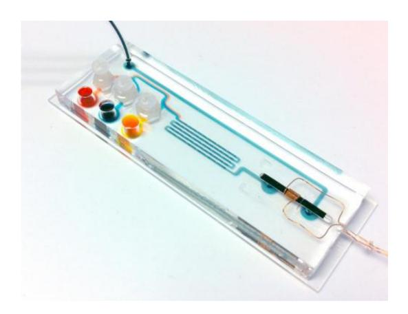
On this 2.5- by 7.5-cm cartridge, DNA extracted from sputum samples is amplified in the chambers on the left. TB-specific sequences are magnetically labeled in the microfluidic mixing channels in the center and detected by passage through the micro-NMR coil on the right. Credit: Center for Systems Biology, Massachusetts General Hospital
