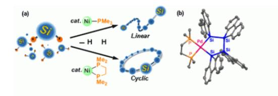
(a) Nickel-catalyzed polymerization to afford linear or cyclic polysilanes and (b) one of possible intermediates in the cyclopolymerization.
