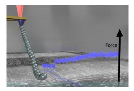
Investigating the friction behavior of nanosystems, scientists from the Technische Universitaet Muenchen (TUM) have discovered a previously unknown type of friction, the so-called desorption stick. They attached a polymer chain to the tip of an AFM and measured the resulting forces while dragging the polymer chain over different surfaces. Credit: B. N. Balzan / TU Muenchen
