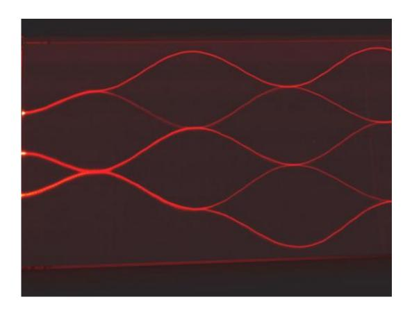
Picture of the optical network – the central part of the Vienna boson sampling computer. According to the laws of quantum physics, the photons seem to take different paths simultaneously as shown in the image. Credit: Philip Walther Group, University of Vienna
