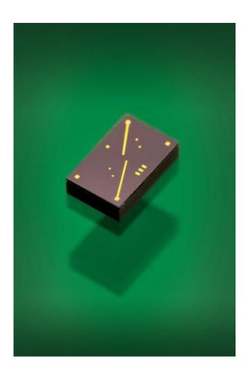
The tiny timing module is a mere 1.5-square millimeters thick. If its frequency fluctuates for any reason, electronic devices could temporarily fail to function properly. Credit: Fraunhofer IZM
