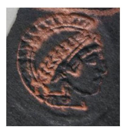
Electrifying Minerva: With the aid of a catalyst, which can be plotted on paper using an inkjet printer, the Potsdam-based researchers converted the symbol of the Max Planck Society into conductive graphite. Amorphous carbon is formed from the non-printed areas of the paper. The scientists then electrolytically coated the graphite Minerva with copper. Credit: MPI of Colloids and Interfaces
