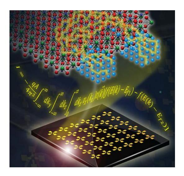
Atomistic diagram for crystalline chromium metal (light blue) on strontium titanate(top), an equation that describes the transport process (middle), and an array of metal contacts on a strontium titanate wafer (bottom). Chambers et al.: Ultra-low Contact Resistance at an Epitaxial Metal/Oxide Heterojunction through Interstitial Site Doping. Advanced Materials. 2013. Credit: Wiley-VCH Verlag GmbH & Co. KGaA
