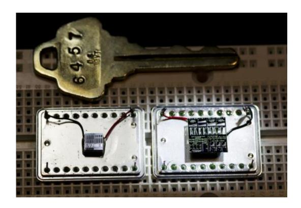
New NIST Reference Materials for MEMS devices are micromachined and further processed to contain miniature cantilevers, beams, stair-like step heights, microscale rulers and test structures for measuring surface-layer thickness. On the left is RM 8096, which was manufactured with an integrated circuit process; on the left is RM 8097, made with a MEMS process. Credit: NIST
