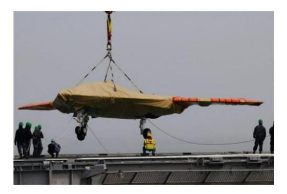
In this image provided by the U.S. Navy an X-47B Unmanned Combat Air System demonstrator is loaded onto the flight deck of the aircraft carrier USS George H.W. Bush on Monday May 6, 2013 in Norfolk, Va. The George H.W. Bush is scheduled to be the first aircraft carrier to catapult launch an unmanned aircraft from its flight deck on Tuesday May 14, 2013. (AP Photo/US Navy, Seaman Joshua P. Card)
