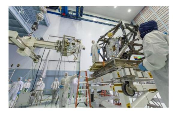
Much like the inside of an operating room, in the clean room at NASA's Goddard Space Flight Center in Greenbelt, MD, engineers worked meticulously to implant part of the eyes of the James Webb Space Telescope. They scrubbed up and suited up to perform one of the most delicate performances of their lives. That part of the eyes, the MIRI, or Mid-Infrared Instrument, will glimpse the formation of galaxies and see deeper into the universe than ever before. Credit: NASA/Chris Gunn
