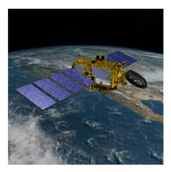
Artist's concept of the U.S./European Jason-3 spacecraft over the California coast. Jason-3 will precisely measure the height of the ocean surface, allowing scientists to monitor ocean circulation and sea level and enabling more accurate weather, ocean and climate forecasts. It will extend the long-term data set established by the Topex/Poseidon, Jason-1 and Jason-2 satellite altimetry missions. The latter two spacecraft are still in operation. Credit: NASA/JPL-Caltech
