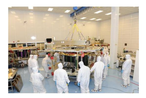
Magnetospheric Multiscale mission integration and test team members, seen here in white clean-room suits, integrate the fourth and final instrument deck onto the spacecraft deck/thrust tube assembly, which houses the propulsion module, officially making it an observatory. This clean room was designed and built for MMS to house all four spacecraft at once: Two additional observatories appear in the background. Credit: NASA
