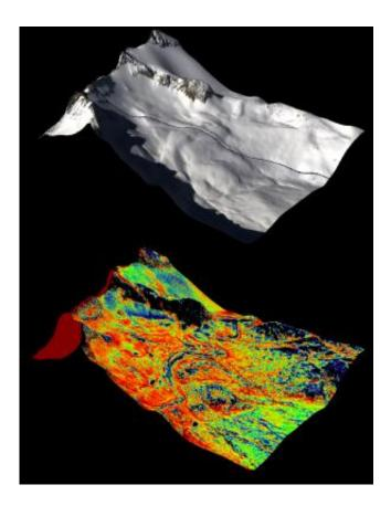
A natural color image of Mt. Lyell, the highest point in the Tuolumne River Basin (top image) is compared with a three-dimensional color composite image of Mt. Lyell from NASA's Airborne Snow Observatory depicting snow depth (bottom image). Mt. Lyell holds the Lyell glacier, which has been in sustained retreat since the 1800s. Credit: NASA JPL/Caltech
