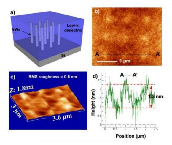
Top surface topography of the low-k dielectric layer that covers the Si NW array using Atomic Force Microscopy (AFM). Credit: *Nanoscale*, 2013,5, 2437-2441.
