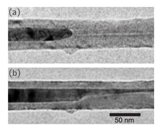
A transmission electron micrograph image of an iron nanocrystal inside a carbon nanotube and the same section after a current has been applied, causing the iron nanoparticle to squeeze into the adjacent constriction. Credit: S. Coh et al., Phys. Rev. Lett. (2013)
