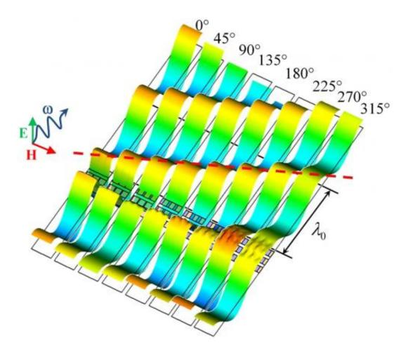
Light propagation through the meta-transmitarray for the eight designs identified in part (d) of the figure above. The phase of the transmitted wave can be shifted from 0 to 360°. Credit: Monticone, et al. American Physical Society ©2013
