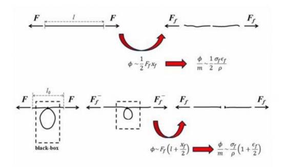
Concept. The classical fibre dissipates during fracture its cumulated strain energy. In contrast, a fibre with a slider, e.g. knot, can dissipate much more energy, thanks to a sliding friction force. Credit: arXiv:1304.6658 [cond-mat.mtrl-sci]
