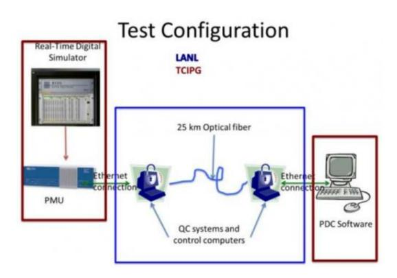
Test configuration using the Los Alamos (LANL) QSC system to secure PMU control commands and data. The TCIPG test bed provided a real-time digital (power) simulator, PMU, and PDC software to control and display data from the PMU. Credit: arXiv:1305.0305 [quant-ph]
