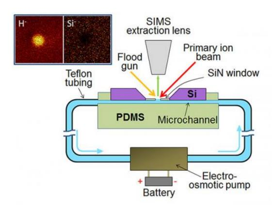
The schematic of a vacuum compatible aqueous SIMS device. Insert shows the secondary H- and Si- ion images of this aperture.
