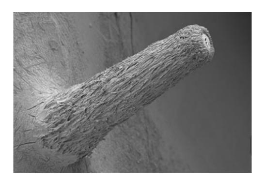
The images were obtained using cryo scanning electron microscopy, where the sample is plunged into liquid nitrogen to freeze it and imaged using the electron microscope.
