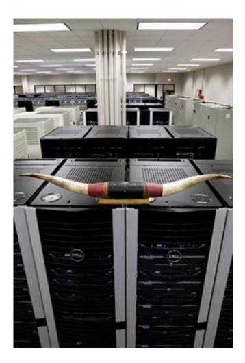
Longhorn, a 256-node Dell visualization cluster, is designed for remote interactive visualization and data analysis. Credit: Texas Advanced Computing Center
