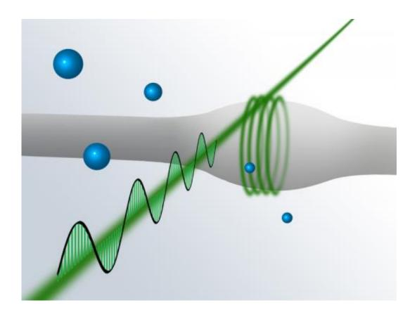
A transversal wave transfers light into a glass fiber, where it is stored in a bottle microresonator. Atoms close to the fiber couple to the light wave.
