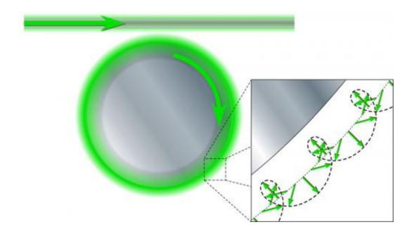
The polarization of the light wave has a longitudinal component - therefore, the polarization direction resembles the tips of the rotor of a flying helicopter, describing a cycloid.
