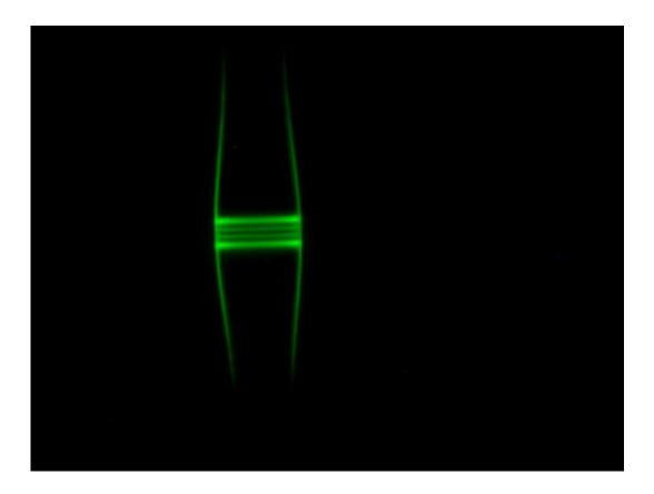
In a glass fiber - with about half the diameter of a human hair - light is kept in place. It cannot escape, because the diameter of the fiber decreases on both sides.
