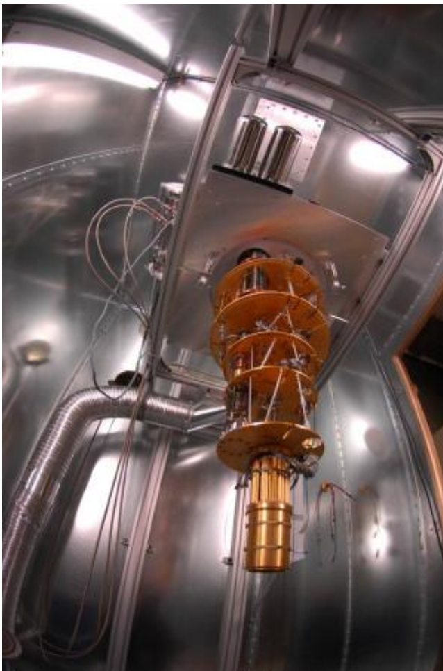
The D-Wave Systems Fridge with Cryogenic Packaging
