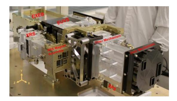
The Extreme Ultraviolet and X-ray Irradiance Sensors (EXIS) detect solar soft X-ray irradiance and solar extreme ultraviolet spectral irradiance in the 5-127 nm range. This is a photo of the EXIS Engineering Test Unit. Credit: NOAA/NASA
