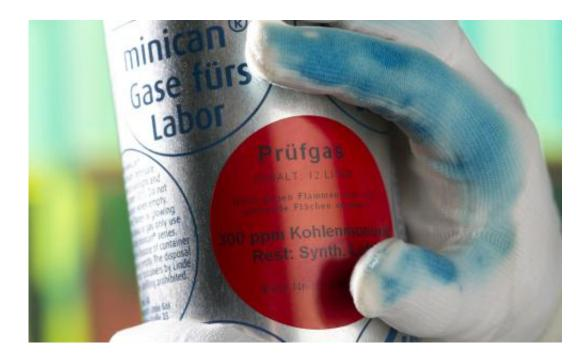
The sensor glove turns blue in the presence of hazardous substances.
