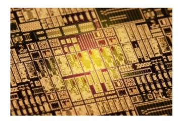
The high frequency chip only measures 4 x 1.5 mm<sup>2</sup>, as the size of electronic devices scales with frequency / wavelength. Credit: Sandra Iselin / Fraunhofer IAF
