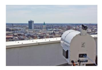
A distance of over one kilometer has already been covered by using a long range demonstrator between two skyscrapers in Karlsruhe. Credit: Ulrich Lewark / KIT
