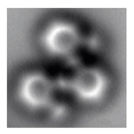
Almost as clearly as a textbook diagram, this image made by a noncontact atomic force microscope reveals the positions of individual atoms and bonds, in a molecule having 26 carbon atoms and 14 hydrogen atoms structured as three connected benzene rings. Credit: Lawrence Berkeley National Laboratory and University of California at Berkeley
