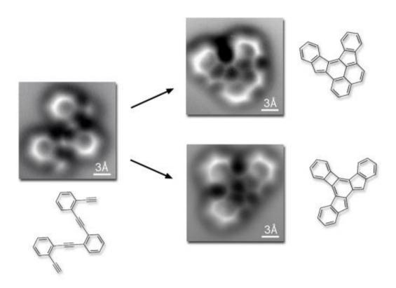
The original reactant molecule, resting on a flat silver surface, is imaged both before and after the reaction, which occurs when the temperature exceeds 90 degrees Celsius. The two most common final products of the reaction are shown. The three-angstrom scale bars (an angstrom is a ten-billionth of a meter) indicate that the reactant and product molecules are about a billionth of a meter across. Credit: Lawrence Berkeley National Laboratory and University of California at Berkeley
