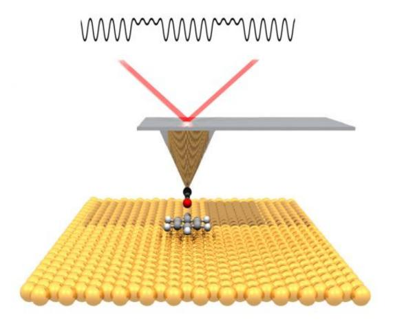
The single-atom tip of the noncontact atomic force microscope "feels" changes in the strength of electronic forces as it moves across the surface at a constant height. Resulting movements of the stylus are detected by a laser beam to compute images. Credit: Lawrence Berkeley National Laboratory and University of California at Berkeley
