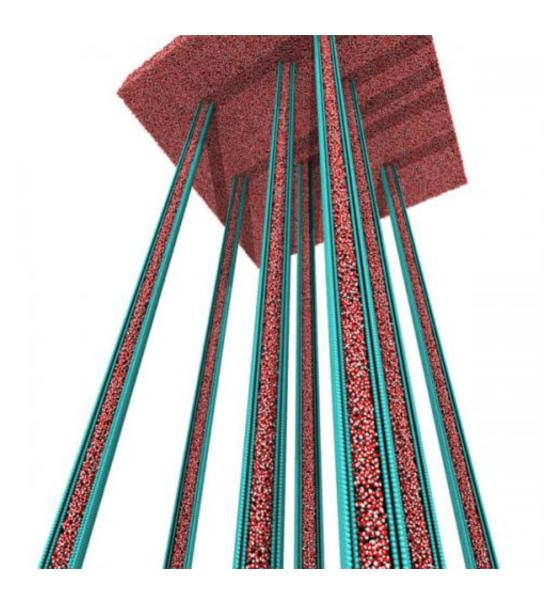
Computer scientists of ETH Zurich simulated the flow of millions of water molecules through long Carbon Nanotubes. Credit: Petros Koumoutsakos / ETH Zurich
