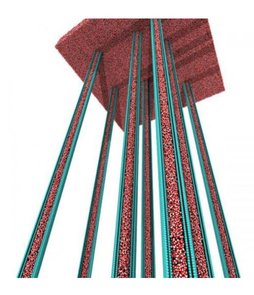
Computer scientists of ETH Zurich simulated the flow of millions of water molecules through long Carbon Nanotubes. Credit: Petros Koumoutsakos / ETH Zurich
