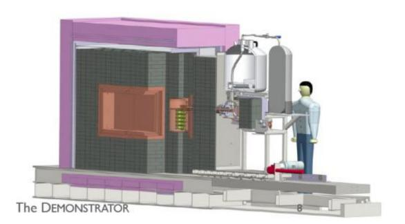
The Majorana Demonstrator is being assembled and stored 4,850 feet beneath the earth's surface in enriched copper to limit the amount of background interference from cosmic rays and radioactive isotopes.
