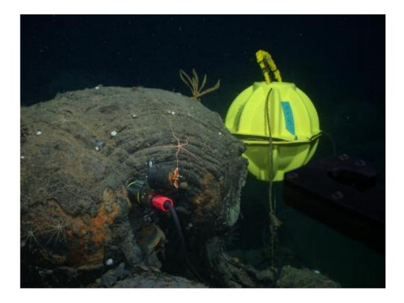
A seismometer was inserted into a hole drilled in seafloor lava. Eight of these instruments were installed at an ocean spreading-center volcano 150 miles off Vancouver Island. A data recording device is enclosed in the yellow sphere. In three years of operation the network detected nearly 40,000 small earthquakes, and hundreds of thousands of fin-whale calls. Credit: John Delaney and Deborah Kelley, UW (taken with remotely operated vehicle Jason)
