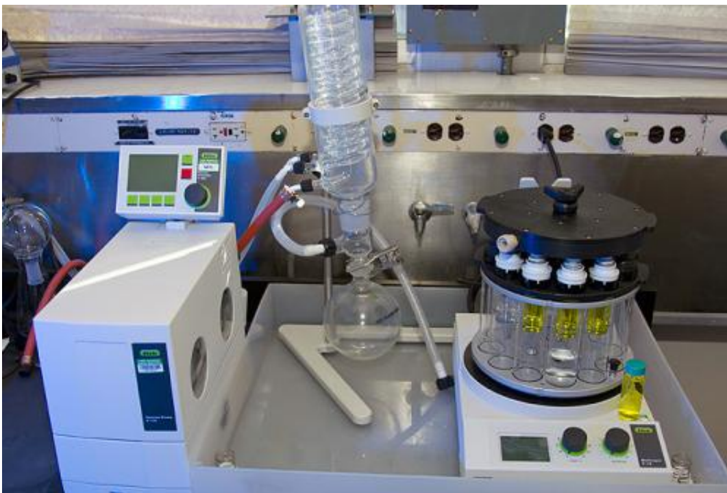
A view of the Buchi Multivapor P-12 Evaporator, apparatus that can be used in the preparation of the uranium sulfate fuel.
