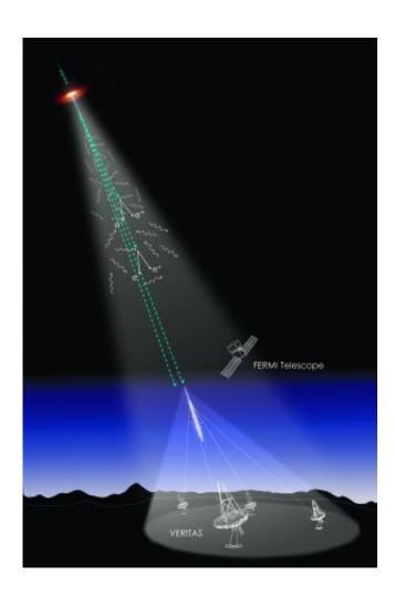
This figure illustrates how energetic gamma rays (dashed lines) from a distant blazar strike photons of extragalactic background light (wavy lines) and produce pairs of electrons and positrons. The energetic gamma rays that are not attenuated by this process strike the upper atmosphere, producing a cascade of charged particles which make a cone of Čerenkov light that is detected by the
