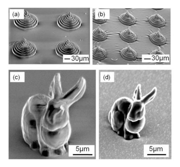
This shows two microstructures made with the new material, containing the highest concentration of RDGE. Left: Pre-charring. These pyramid and bunny models did not respond to the preferred method of 3-D shaping, so they were created using an alternative process. Right: Post-charring. Notice that the pyramid and bunny shrink significantly less than those made from the material with a lower concentration of RDGE. Credit: Optical Materials Express
