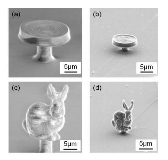
This shows two microstructures made with the new material, containing the lowest concentration of RDGE. Left: Pre-carbonization. This circular table and bunny models, just slightly larger than a typical bacterium, were formed using two-photon polymerization, the preferred method of 3-D shaping. Right: The same models after they have been carbonized, or charred. Notice that they shrink
