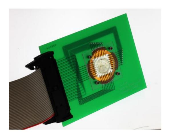
The new digital cameras exploit large arrays of tiny focusing lenses and miniaturized detectors in hemispherical layouts, just like eyes found in arthropods. Full 180 degree fields of view with zero aberrations can only be
