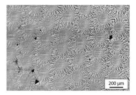
Cross-section of the new tungsten compound. The microscope shows the circular cross-sections of hair-fine tungsten wires, tightly bunched and embedded in a tungsten matrix. Credit: IPP, Johann Riesch
