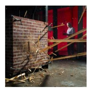
Texas Tech researchers use the wind cannon to determine how certain building materials withstand debris being lauched at various speeds.
