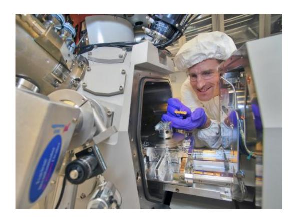
CFN's Kim Kisslinger, seen here with a focused-ion beam instrument, reduced the InGaN samples to a thickness of just 20 nanometers to prepare them for electron microscopy.
