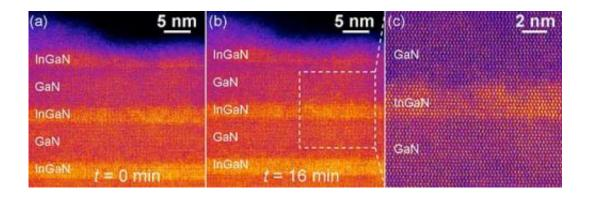
These images of the InGaN samples—produced by CFN's low-voltage scanning transmission electron microscope—reveal a lack of structural changes over time. After 16 minutes of scanning, no damage or decomposition is visible, and the higher magnification (c) exhibits none of the clustering previously theorized to be central to LED efficiency.
