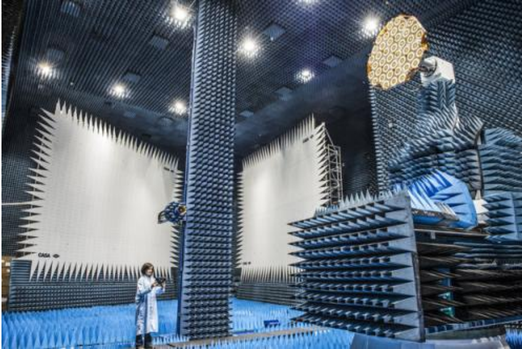
Compact Payload Test Range for antenna testing.
