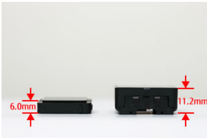
Figure 2: Comparison of new (left) and conventional (right) sensors.
