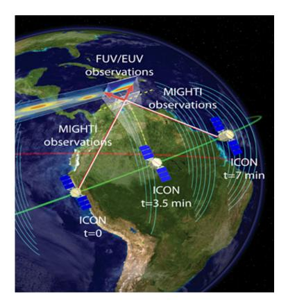
The ICON satellite will orbit Earth at a 27 degree angle to the equator, pointing its MIGHTI imager and far and extreme ultraviolet sensors at ionospheric storms as on-board instruments measure the flow of charged-particles (guided by the arched magnetic field shown with blue lines) at the position of the satellite.
