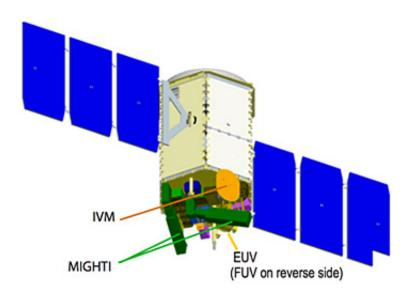
The ICON spacecraft, with blue solar panels and limb-pointing instruments to measure winds in the thermosphere (MIGHTI), far and extreme ultraviolet emissions (FUV and EUV) from the ionosphere and the in situ ion velocity meter (IVM).
