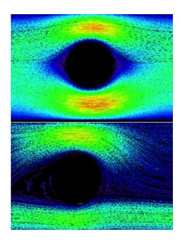
Data from the experiment, showing laminar (top) and turbulent (flow) flow around the posts at the beginning of the pipe.
