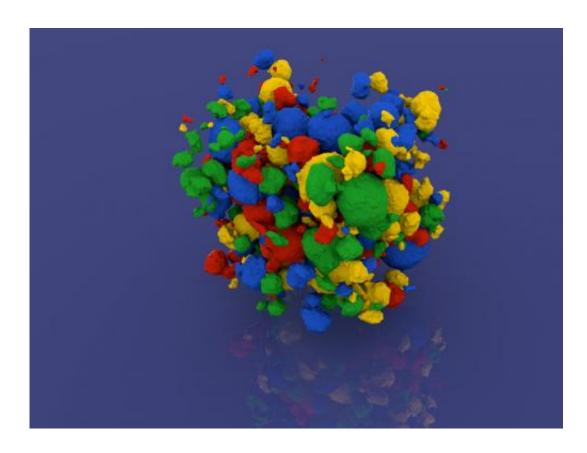
Electrodes of Lithium ion batteries are composed of various particles of different shapes and sizes. These particles have a strong influence on how fast ions flow through the electrode. Credit: Martin Ebner / ETH Zurich
