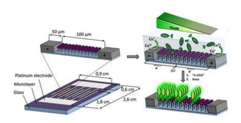
Dutch nanotechnologists at the University of Twente's MESA+ research institute have developed a tiny chip that makes it easy to create micrometre scale gradients. Gradients are gradual transitions in specific properties, such as acidity. This newly-developed system can be used to efficiently measure the reaction kinetics of various chemical or biological reactions. The results of this research work will be published in the scientific journal *Nature Communications*, on April 9.
