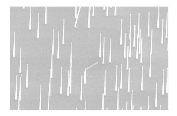
This Scanning Electron Microscope image shows an array of nanowires. Credit: Kristian Molhave/Opensource Handbook of Nanoscience and Nanotechnology
