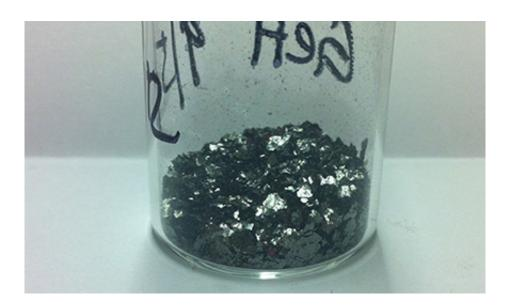
The element germanium in its natural state. Researchers at The Ohio State University have developed a technique for making one-atom-thick sheets of germanium for eventual use in electronics. Credit: Joshua Goldberger, The Ohio State University
