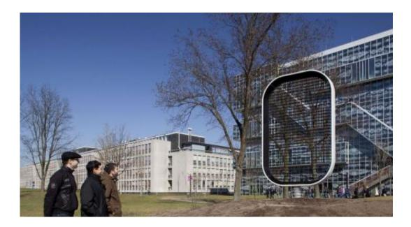
(Phys.org) —Faculty members at Delft University in the Netherlands have teamed up with architectural firm Mecanoo to develop a new way to generate electricity using wind energy. The result is the Electrostatic WInd-energy CONvertor, (EWICON)—a windmill with no moving mechanical parts. Its creators say that it makes no noise, won't break down or cast a shadow and it won't cause bird deaths—all problems associated with traditional wind turbines.
