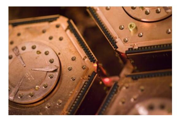
The Cryogenic Dark Matter Search experiment uses five towers of dark matter detectors like the ones shown here. Credit: Fermilab
