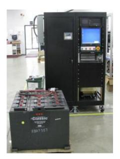
An Exide forklift truck battery being charged using the rapid charging system. Credit: Potential Difference Inc.
